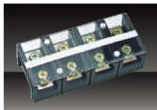
TC-2004 Wire range:100mm 2 Rated current/Voltage:200A/600V
