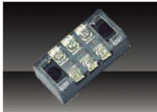
TB-2503 Wire range:0.5-2.5mm 2 Rated current/Voltage:25A/600V
