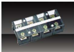
TC-604 Wire range:14mm 2 Rated current/Voltage:60A/600V
