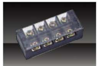
TB1004 Wire range:0.5-2.5mm 2 Rated current/Voltage:100A/600V
