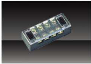
TB-1504 Wire range:0.5-1.5mm 2 Rated current/Voltage:15A/600V
