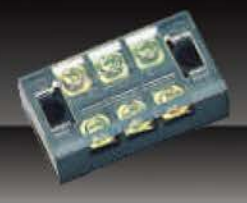
TB-4503 Wire range:0.5-4mm 2 Rated current/Voltage:45A/600V
